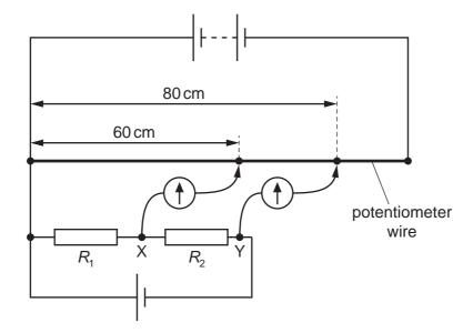
One terminal of a galvanometer is connected to point X. The galvanometer reads zero when its other terminal is connected to a point that is a distance of 60 cm from one end of the potentiometer wire.
