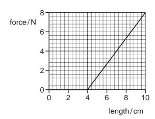
The graph shows the variation with length of the force applied to **one** of the springs.
