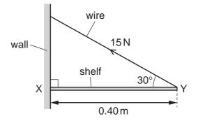
The tension force in the wire is 15 N at an angle of 30° to the horizontal.
